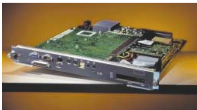
ACCELERATED MONITORING: Integrating intrusion detection into the Catalyst 6000 switch overcomes the limitations of using SPAN ports. The capability of running as many as eight modules, for example, enables the switch to monitor traffic at gigabit-per-second speeds.
